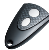
Micro-Novotron 512 Design 2-kanaals, 433 MHz, rolling code (KeeLoq)
